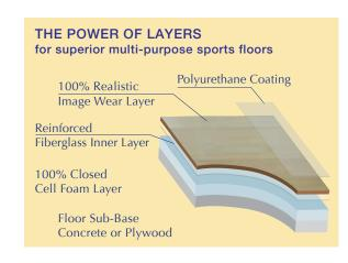
ElastiFlex is also available in thicknesses of 5/16" and 3/16" on a special order basis.
